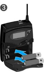
▶ Close the battery compartment.The cover locks into place with an audible click.
