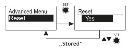
When you reset the bodypack transmitter, only the selected settings of the pilot tone and the  ${\bf U}$  frequency bank are retained.
