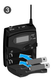
▶ Close the battery compartment.The cover locks into place with an audible click.
